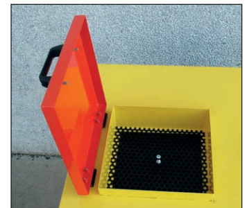
Chamber of drain used filters
