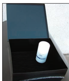
Chamber of drain used filters
