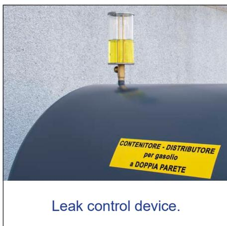
Leak control device.
